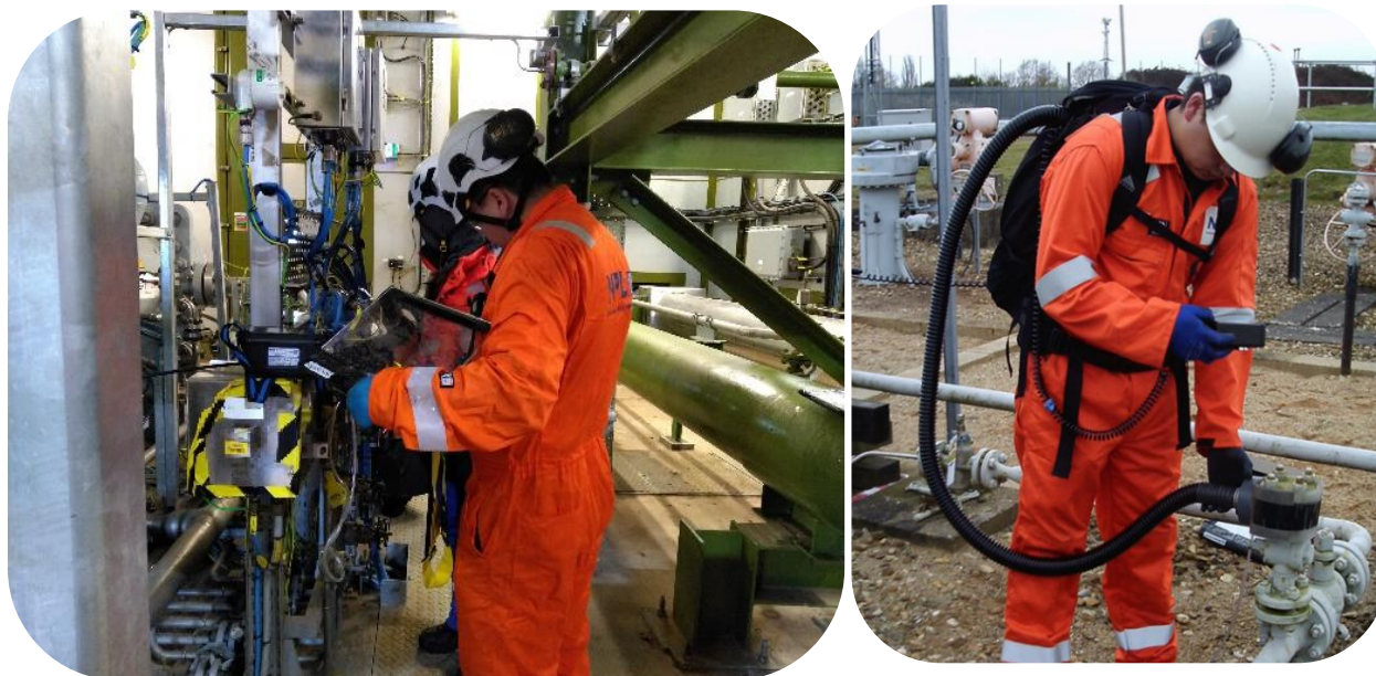
A portable sniffer for detecting methane leaks, left , and a portable high flow sampler for quantifying methane emissions, right . Both capabilities at NPL, soon to be developed for hydrogen
