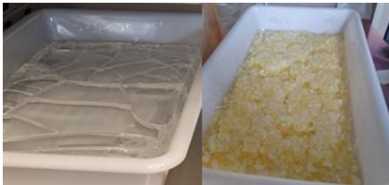
Figure 3: A tray of the solid material as it gels (left) and then dries (right).
