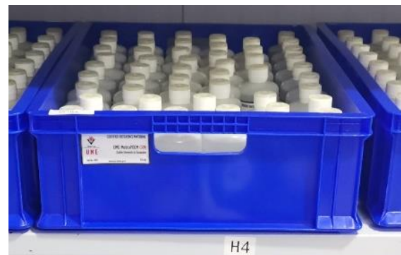
Figure 6: The candidate Seawater CRM batch of 470 bottles which are stored at +4 °C
