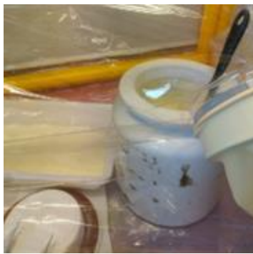
Figure 4: Handling of the material in a disposable glovebox after jar milling
