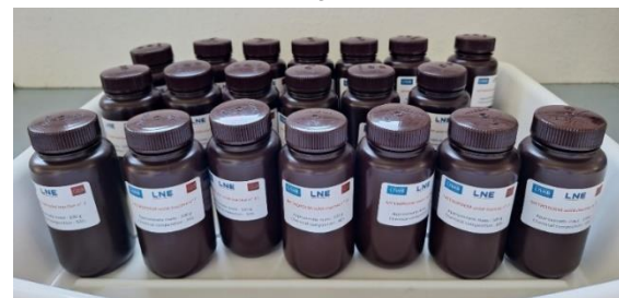
Figure 3: Picture of the batch of 20 samples of inactive solid reference material produced.
