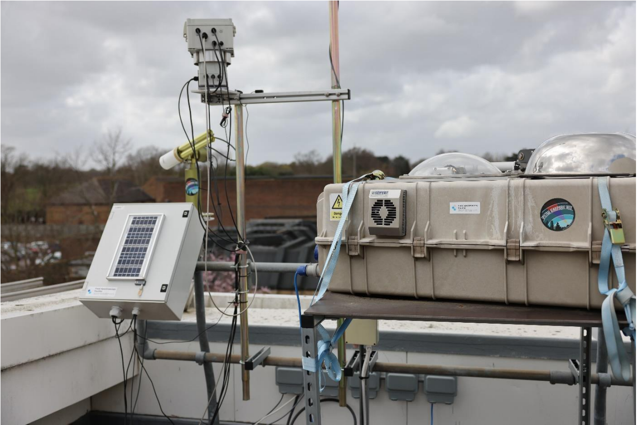
Image 11: GEMMA equipment measuring greenhouse gases and urban pollutants in the atmosphere
