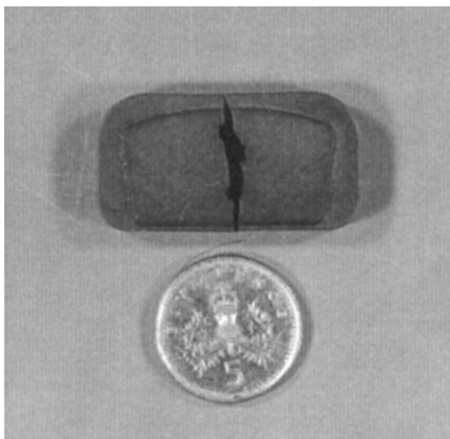
Figure A.4.3 - Gas valve plate (a) which has fractured into two pieces across the series of gas passage holes, with evidence of missing fragments.
